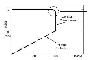
Typical LED power supply I-V curve
