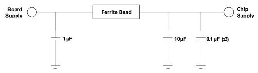
Figure 19. Power Supply Decoupling
