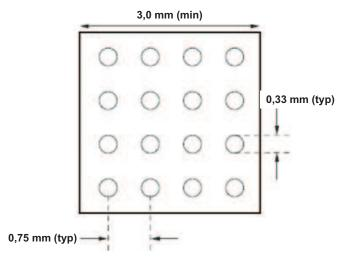
Figure 20. Recommended PCB Layout
