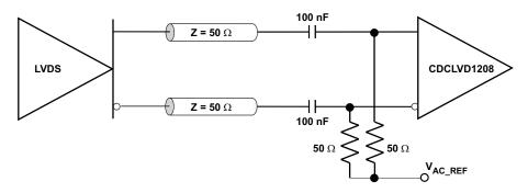
Figure 13. LVDS Clock Driver Connected to CDCLVD1208 Input (AC-Coupled)
