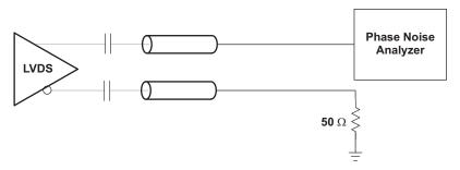
Figure 4. LVDS Output AC Configuration During Device Test
