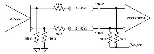
Figure 14. LVPECL Clock Driver Connected to CDCLVD1208 Input
