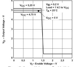
Figure 7. Output Voltage vs Enable Voltage
