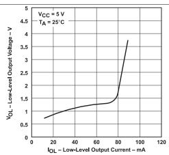
Figure 2. Driver, Low-Level Output Voltage vs
