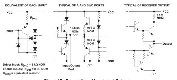
Figure 15. Schematics of Inputs and Outputs
