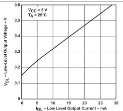
Figure 4. Receiver, Low-Level Output Voltage vs
