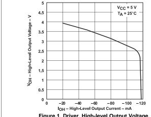
Figure 1. Driver, High-level Output Voltage vs
