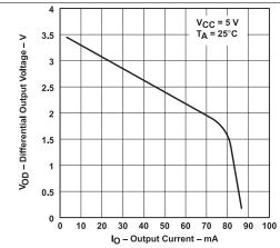
Figure 3. Driver, Differential Output Voltage vs
