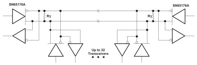
The line should be terminated at both ends in its characteristic impedance ( $R_T = Z_O$ ). Stub lengths off the main line should be kept as short as possible.
