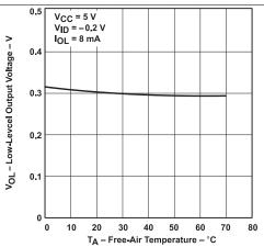
Figure 5. Receiver, Low-Level Output Voltage vs
