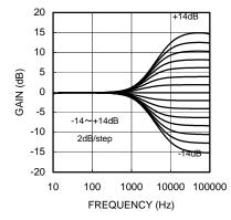
Fig.8 Treble gain - Frequency
