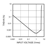
Fig.6 THD+N - Input voltage
