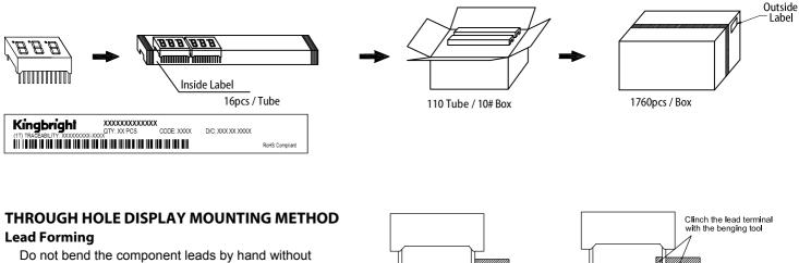
proper tools. The leads should be bent by clinching the upper part of the lead firmly such that the bending force is not exerted on the plastic body.
