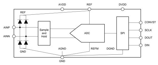
Figure 45. Detailed Block Diagram
