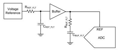
Figure 48. Reference Driver Schematic
