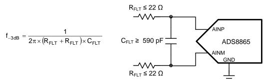
Figure 69. Antialiasing Filter
