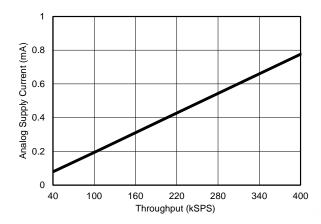
Figure 66. Power Scaling with Throughput
