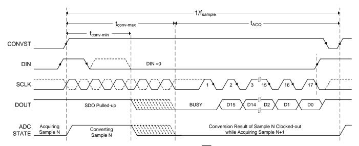
Figure 59. Interface Timing Diagram: 4-Wire CS Mode With a Busy Indicator
