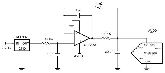
Figure 68. Schematic of Reference Driver Circuit with  $V_{REF} = 2.5 \text{ V DC}$
