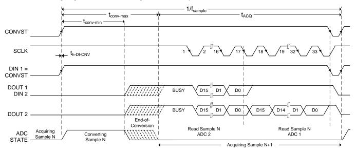
Figure 63. Interface Timing Diagram: For Two Devices in Daisy-Chain Mode With a Busy Indicator
