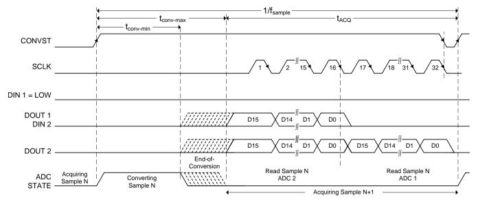
Figure 61. Interface Timing Diagram: For Two Devices in Daisy-Chain Mode Without a Busy Indicator
