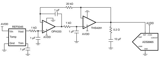
Figure 67. Schematic of Reference Driver Circuit with  $V_{REF} = 4.5 V$
