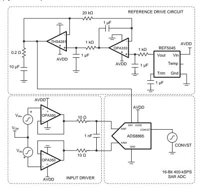
Figure 70. DAQ Circuit for 2.5-µs, Full-Scale Step Response
