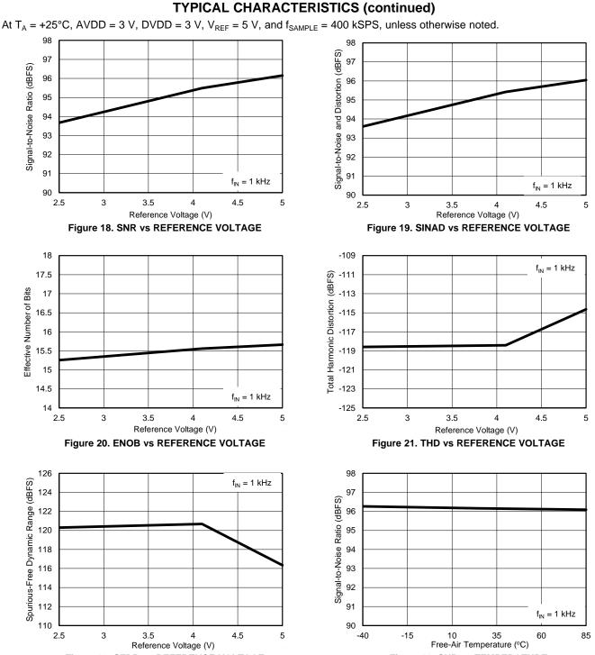
Figure 22. SFDR vs REFERENCE VOLTAGE
