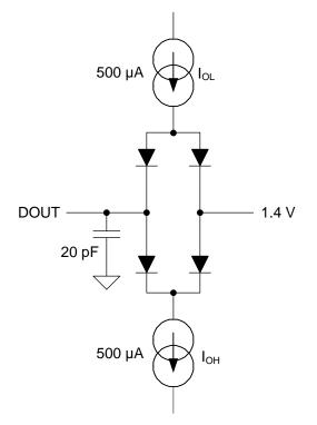
Figure 4. Load Circuit for Digital Interface Timing
