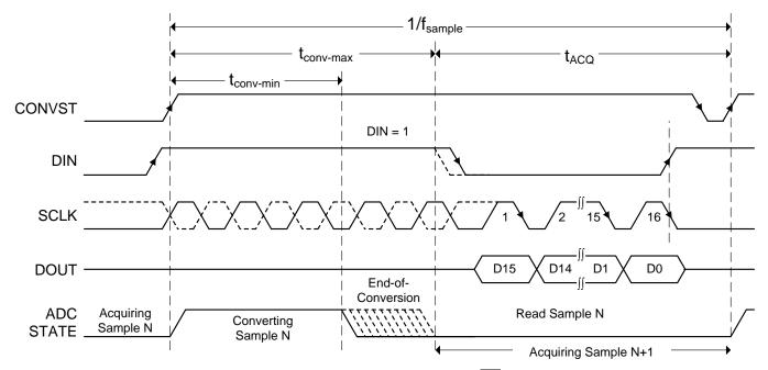
Figure 55. Interface Timing Diagram: Single ADC with 4-Wire CS Mode Without a Busy Indicator
