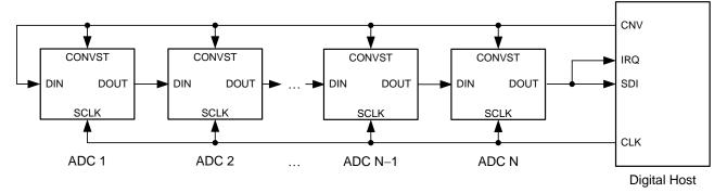
Figure 62. Connection Diagram: Daisy-Chain Mode With a Busy Indicator (DIN = 0)
