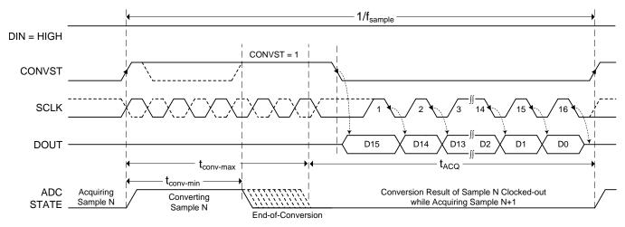
Figure 51. Interface Timing Diagram: 3-Wire CS Mode Without a Busy Indicator (DIN = 1)
