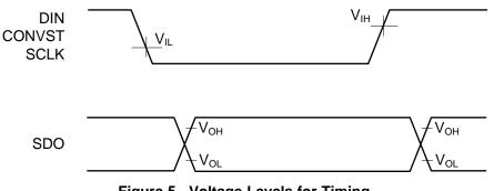
Figure 5. Voltage Levels for Timing
