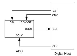
Figure 54. Connection Diagram: Single ADC with 4-Wire CS Mode Without a Busy Indicator
