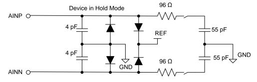
Figure 47. Input Sampling Stage Equivalent Circuit
