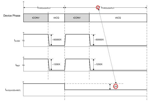
Figure 65. Power Scaling with Throughput
