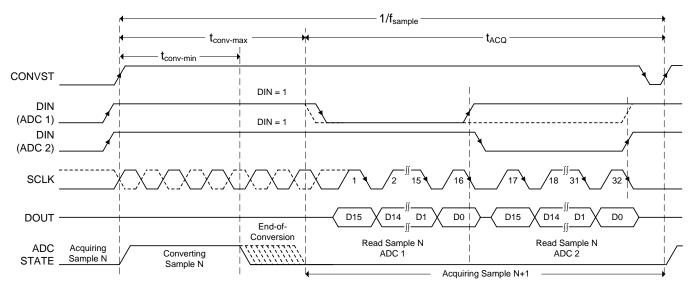
Figure 57. Interface Timing Diagram: Two ADCs with 4-Wire CS Mode Without a Busy Indicator
