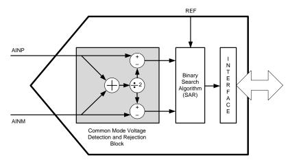
Figure 46. Conceptual Diagram: True Differential Input Structure
