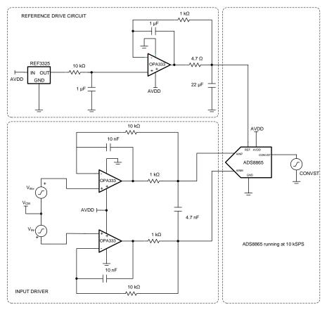
Figure 74. Ultralow-Power DAQ Circuit at 10 kSPS
