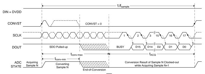
Figure 53. Interface Timing Diagram: 3-Wire  $\overline{CS}$  Mode With a Busy Indicator (DIN = 1)
