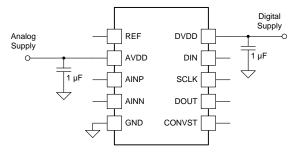
Figure 64. Supply Decoupling
