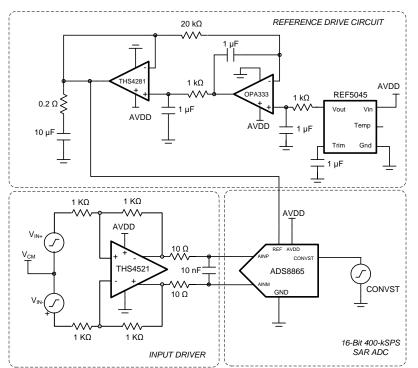
Figure 72. Differential Input DAQ Circuit for Lowest Distortion and Noise at 400 kSPS
