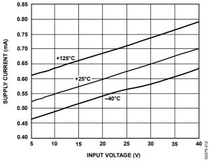
Figure 12. REF03 Supply Current vs. Input Voltage
