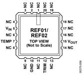
Figure 6. 20-Terminal LCC (RC-Suffix) Pin Configuration
