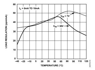
Figure 15. REF03 Load Regulation vs. Temperature
