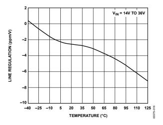
Figure 16. REF01 Line Regulation vs. Temperature
