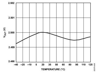
Figure 9. REF03 Typical Output Voltage vs. Temperature
