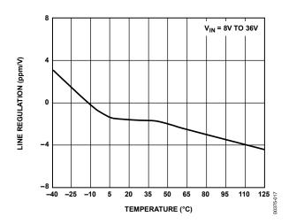
Figure 17. REF02 Line Regulation vs. Temperature
