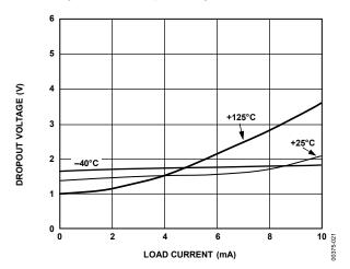
Figure 21. REF03 Dropout Voltage vs. Load Current
