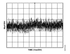
Figure 24. REF02 Typical Wideband Voltage Noise (10 Hz to 10 kHz)
