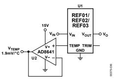
Figure 36. Temperature Monitoring
