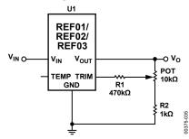
Figure 35. Optional Trim Adjustment Circuit
