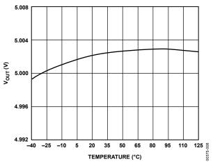
Figure 8. REF02 Typical Output Voltage vs. Temperature
