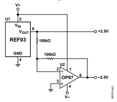
Figure 42. Bipolar Voltage Reference
