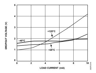
Figure 19. REF01 Dropout Voltage vs. Load Current
