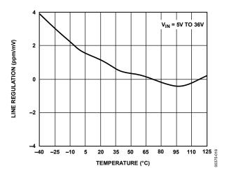
Figure 18. REF03 Line Regulation vs. Temperature
