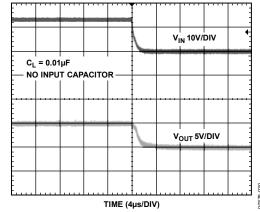
Figure 30. REF02 Turn-Off Response (No Input Capacitor)
