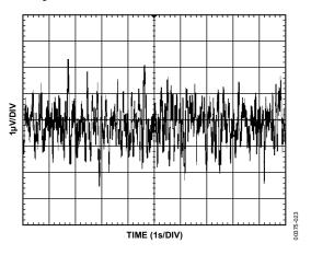
Figure 23. REF02 Typical Low-Frequency Voltage Noise (0.1 Hz to 10.0 Hz)
