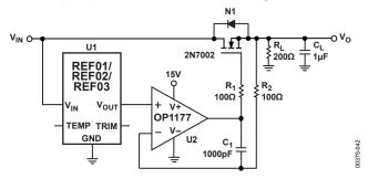
Figure 41. Precision Boosted Output Regulator
