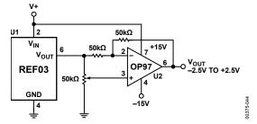
Figure 43. Negatively Adjustable Reference
