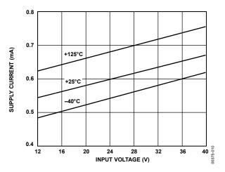
Figure 10. REF01 Supply Current vs. Input Voltage
