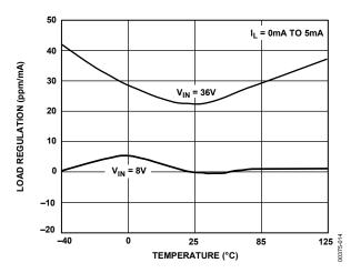
Figure 14. REF02 Load Regulation vs. Temperature
