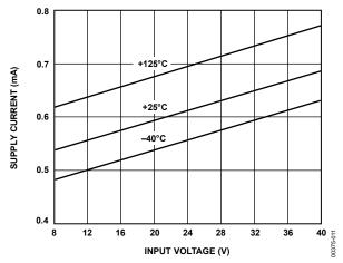
Figure 11. REF02 Supply Current vs. Input Voltage
