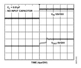
Figure 31. REF02 Turn-Off Response (No Input Capacitor)
