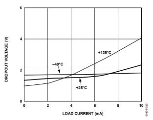
Figure 20. REF02 Dropout Voltage vs. Load Current
