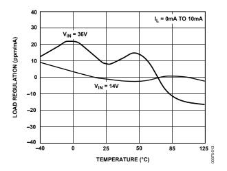
Figure 13. REF01 Load Regulation vs. Temperature
