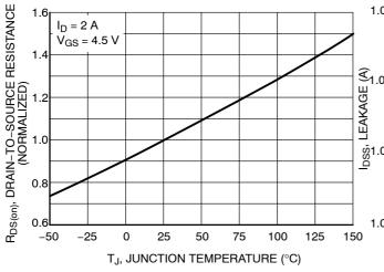
Figure 5. On–Resistance Variation with Temperature
