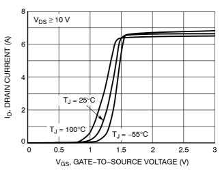
Figure 2. Transfer Characteristics
