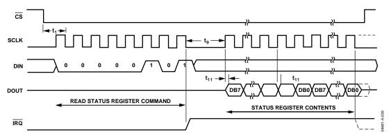
Figure 38. Interrupt Timing
