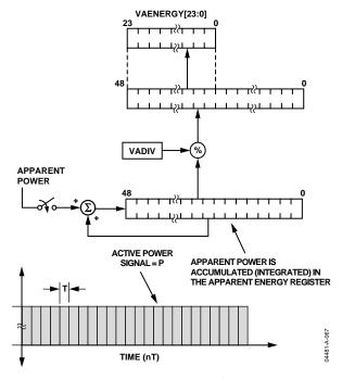
Figure 66. Apparent Energy Calculation
