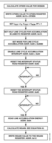
Figure 72. Calibrating Watt Gain Using an Accurate Source
