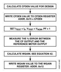
Figure 71. Calibrating Watt Gain Using a Reference Meter
