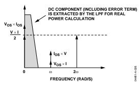
Figure 25. Effect of Channel Offsets on the Real Power Calculation
