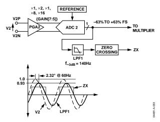
Figure 32. Zero-Crossing Detection on Channel 2
