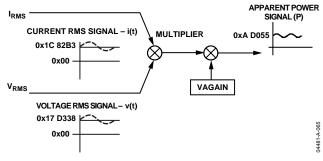
Figure 64. Apparent Power Signal Processing
