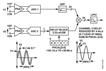
Figure 49. Phase Calibration
