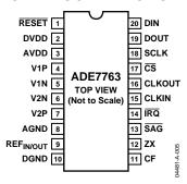
Figure 5. Pin Configuration (SSOP Package)
