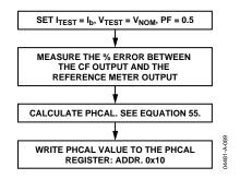
Figure 75. Calibrating Phase Using a Reference Meter
