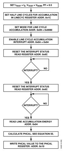
Figure 76. Calibrating Phase with an Accurate Source
