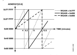
Figure 58. Energy Register Rollover Time for Full-Scale Power (Minimum and Maximum Power Gain)
