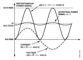
Figure 53. Active Power Calculation
