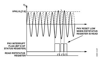
Figure 36. Peak Level Detection
