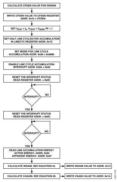
Figure 78. Active/Apparent Gain Calibration
