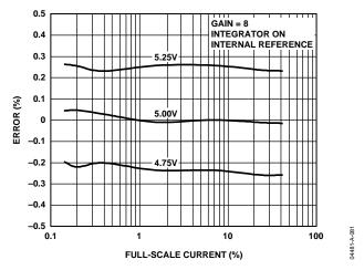
Figure 18. Active Energy Error as a Percentage of Reading (Gain = 8) over Power Supply with Internal Reference and Integrator On
