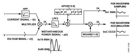
Figure 57. Active Power Signal Processing
