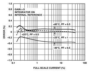
Figure 15. Active Energy Error as a Percentage of Reading (Gain = 8) over Power Factor with Internal Reference and Integrator On
