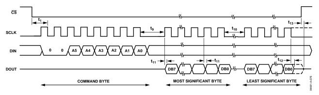
Figure 85. Serial Interface Read Timing
