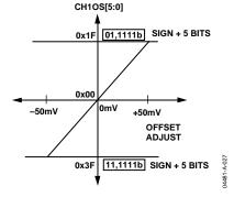
Figure 26. Channel 1 Offset Correction Range (Gain = 1)
