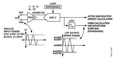
Figure 47. ADC and Signal Processing in Channel 2
