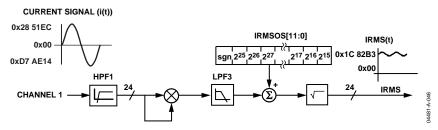
Figure 45. Channel 1 RMS Signal Processing
