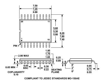
Figure 89. 20-Lead Shrink Small Outline Package [SSOP] (RS-20)
