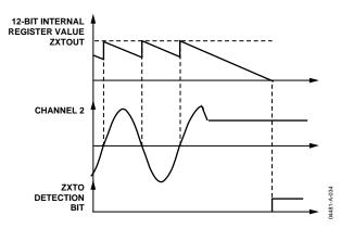
Figure 33. Zero-Crossing Timeout Detection
