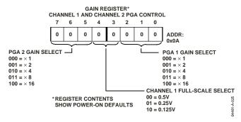
Figure 24. Analog Gain Register
