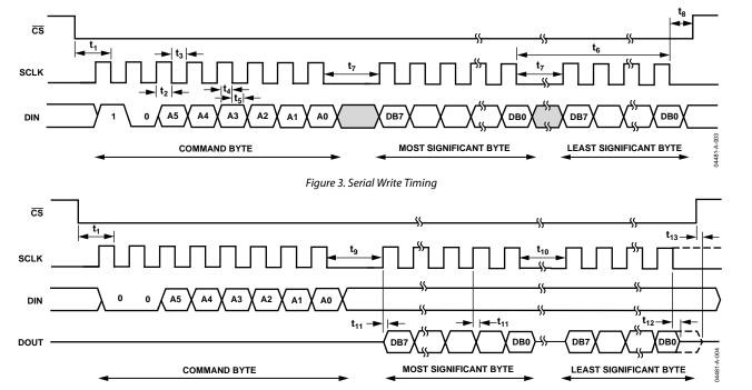
Figure 4. Serial Read Timing
