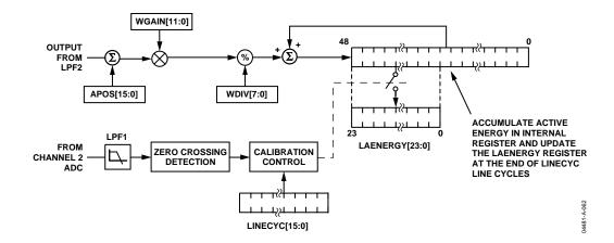
Figure 61. Energy Calculation Line Cycle Energy Accumulation Mode
