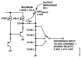
Figure 42. Reference Circuit Output
