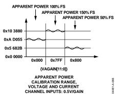
Figure 65. Apparent Power Calculation Output Range
