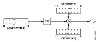
Figure 59. Energy-to-Frequency Conversion
