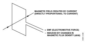
Figure 27. Principle of a di/dt Current Sensor
