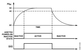
Figure 34. On-Chip Power Supply Monitor
