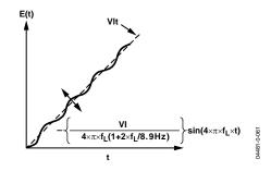
Figure 60. Output Frequency Ripple
