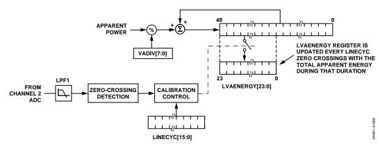
Figure 68. Apparent Energy Calibration
