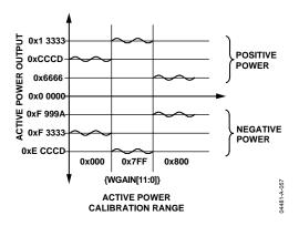
Figure 56. Active Power Calculation Output Range
