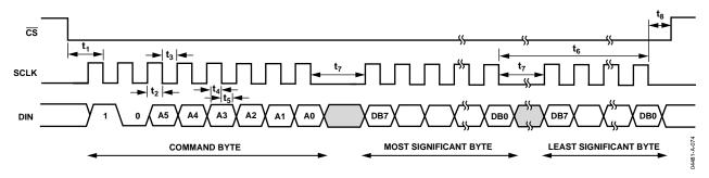
Figure 83. Serial Interface Write Timing
