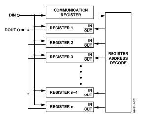
Figure 80. Addressing ADE7763 Registers via the Communication Register
