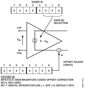
Figure 23. PGA in Channel 1
