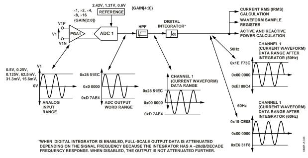
Figure 43. ADC and Signal Processing in Channel 1
