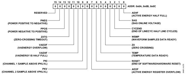
Figure 87. Interrupt Status/Interrupt Enable Register
