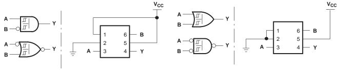
Figure 3. 2-Input AND Gate With Inverted B Input
