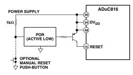
Figure 48. External Active Low POR Circuit
