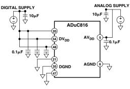
Figure 49. External Dual Supply Connections
