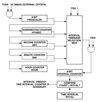
Figure 31. TIC, Simplified Block Diagram
