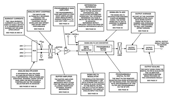
Figure 18. Primary ADC Block Diagram
