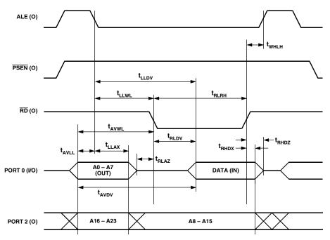
Figure 4. External Data Memory Read Cycle
