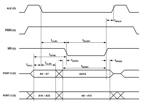
Figure 5. External Data Memory Write Cycle
