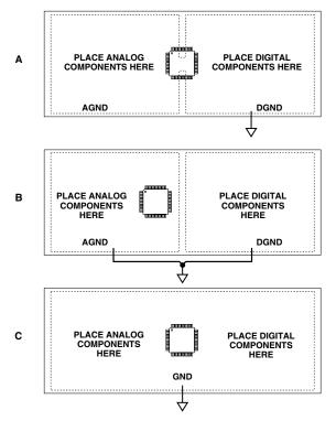
Figure 51. System Grounding Schemes
