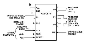
Figure 28. Flash/EE Memory Parallel Programming
