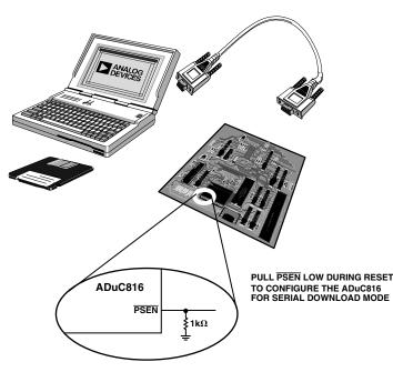
Figure 27. Flash/EE Memory Serial Download Mode Programming
