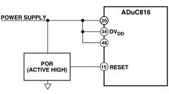
Figure 47. External Active High POR Circuit
