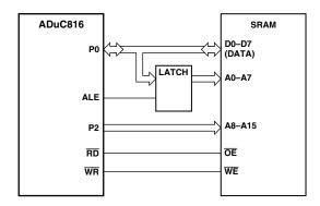
Figure 44. External Data Memory Interface (64 K Address Space)
