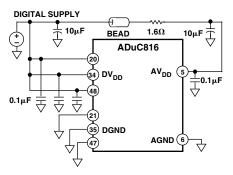
Figure 50. External Single Supply Connections
