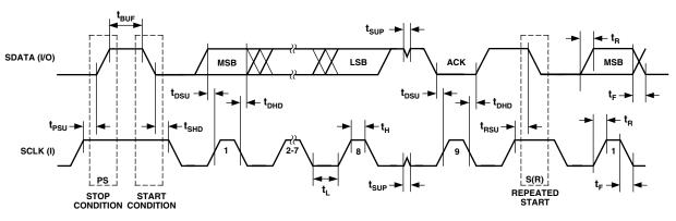
Figure 7. I<sup>2</sup>C-Compatible Interface Timing
