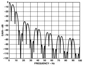
Figure 22. Filter Response, SF = 255 dec
