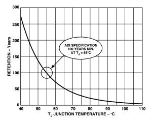
Figure 26. Flash/EE Memory Data Retention
