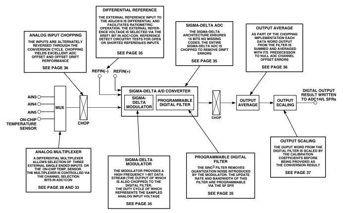
Figure 19. Auxiliary ADC Block Diagram
