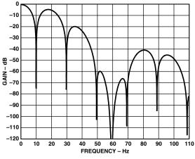
Figure 21. Filter Response, SF = 69 dec
