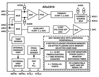
intended for the measurement of wide dynamic range, low frequency signals, such as those in weigh scale, strain gauge, pressure transducer, or temperature measurement applications. The ADC output data rates are programmable and the ADC output resolution will vary with the programmed gain and output rate.
