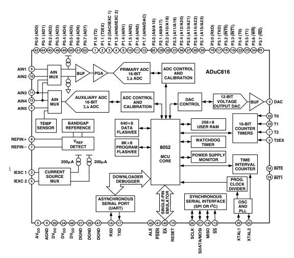
Figure 12. Block Diagram
