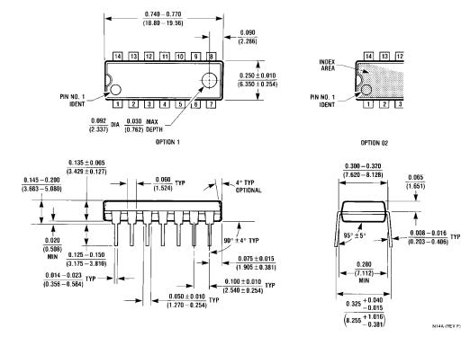
14-Pin Molded Dual-In-Line Package (N)
