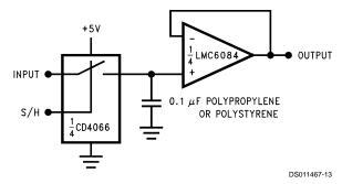
FIGURE 8. Low-Leakage Sample and Hold
