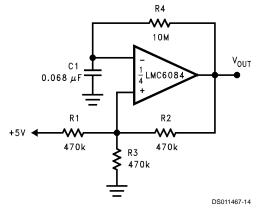
FIGURE 9. 1 Hz Square Wave Oscillator
