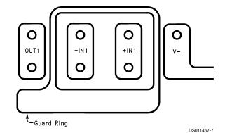
FIGURE 4. Example of Guard Ring in P.C. Board Layout
