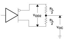
Figure 1. Driver  $V_{OD2}$  and  $V_{OC}$
