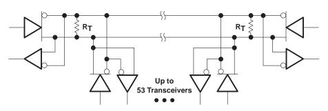
NOTE A: The line should terminate at both ends in its characteristic impedance (R<sub>T</sub> = Z<sub>O</sub>). Stub lengths off the main line should be kept as short as possible.
