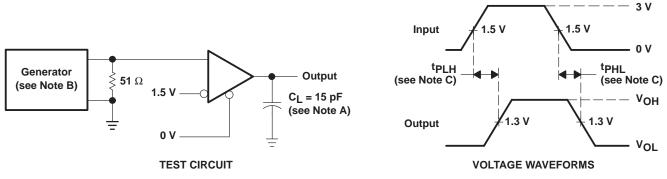
NOTES: A. C<sub>1</sub> includes probe and jig capacitance.
