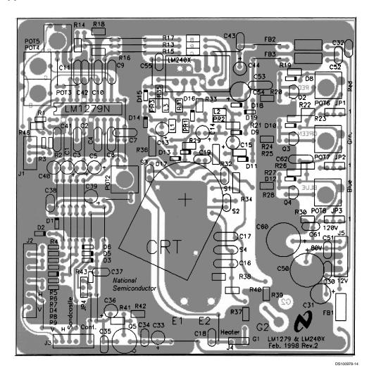
FIGURE 11. LM1279/240X Demo Board Layout
