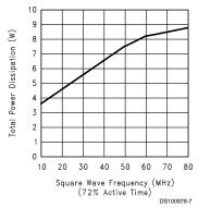
FIGURE 6. Power Dissipation vs Frequency
