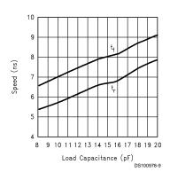
FIGURE 8. Speed vs Load Capacitance
