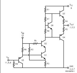
FIGURE 1. Simplified Schematic Diagram (One Channel)
