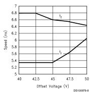
FIGURE 7. Speed vs Offset
