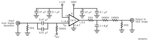
Note: 8 pF load includes parasitic capacitance.
