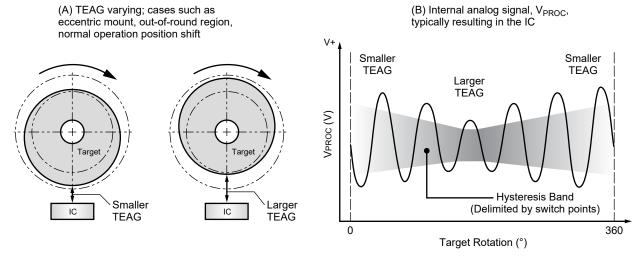
(C) Referencing the internal analog signal,  $V_{\mbox{\footnotesize{PROC}}}$ , to continuously update device response
