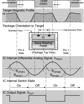
Figure 3. The magnetic profile reflects the geometry of the target, allowing the ATS667 to present an accurate digital output response.
