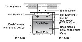
Figure 1. Relative motion of the target is detected by the dual Hall elements mounted on the Hall IC.
