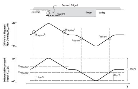
aSensed Edge: leading (rising) mechanical edge in forward rotation, trailing (falling) mechanical edge in reverse rotation
