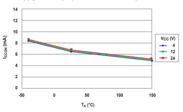
Supply Current (On) versus Supply Voltage
