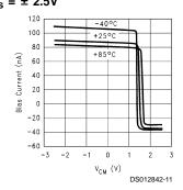
Non Inverting Input, **Bias Current vs Common Mode Voltage**
