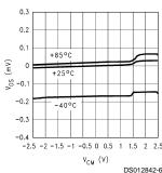
$V_{OS}$  vs  $V_{CM}$  $V_{S} = \pm 15V$
