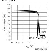
Non Inverting Input, **Bias Current vs Common Mode Voltage**  $V_S = \pm 2.5V$
