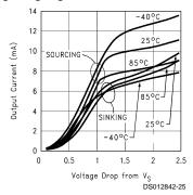
**Short Circuit Current** vs Supply Voltage
