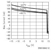
Inverting Input, **Bias Current vs Common Mode Voltage**
