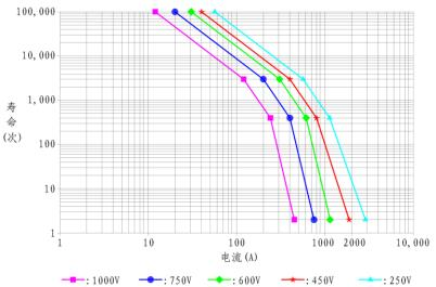
Note: Except for special note, the ambient temperature of electrical durability test is 23  $^{\circ}$ C, and the on-break ratio is: 1s: 9s
