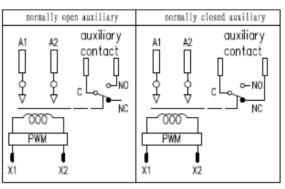
schematic: no polarity requirement for each contact
