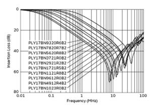
Common Mode Insertion Loss-Frequency Characteristics
