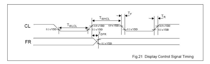
CL and FR timing characteristics at VDD=5 volts
