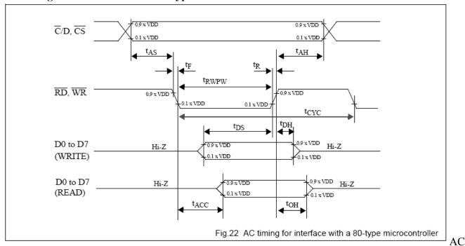
timing for interface with a 80-type microcontorller at VDD=5 volts VDD = 5 V  $\pm 10\%$ ; VSS = 0 V; Tamb = -20 °C to +75°C.
