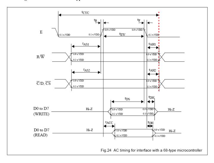
AC timing for interface with a 68-type microcontroller at VDD=5 volts VDD = 5 V  $\pm 10\%$ ; VSS = 0 V; Tamb = -20 °C to +75 °C.
