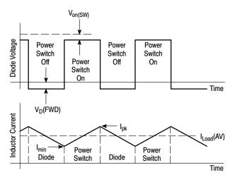
Figure 16. Buck Converter Idealized Waveforms
