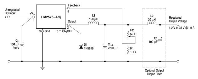
Figure 33. Adjustable Power Supply with Low Ripple Voltage
