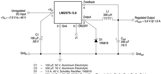
L1 - 330  $\mu$ H, Tech 39: 77 458 BV, Toroid Core, Through–Hole, Pin 3 = Start, Pin 7 = Finish
