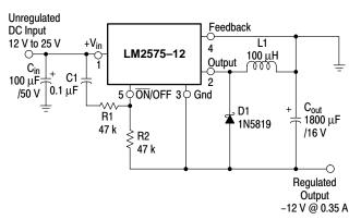
Figure 26. Inverting Buck-Boost Regulator with Delayed Startup
