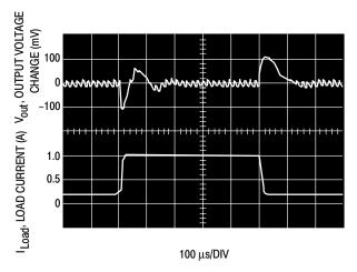
**Figure 13. Load Transient Response**
