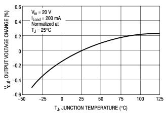
**Figure 2. Normalized Output Voltage**
