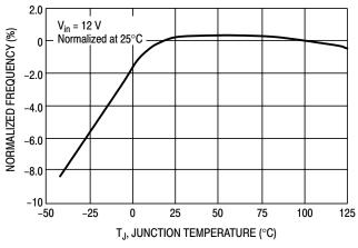
Figure 10. Oscillator Frequency
