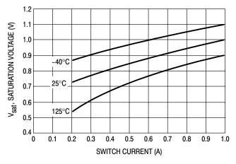
Figure 4. Switch Saturation Voltage
