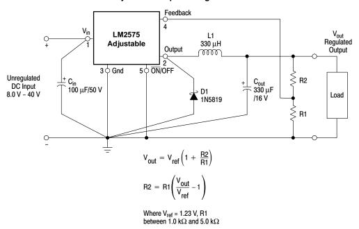
Figure 14. Typical Test Circuit
