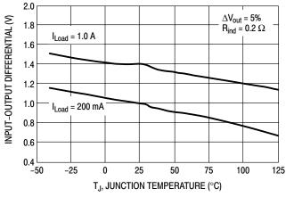
Figure 6. Dropout Voltage
