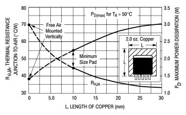
Figure 34. D<sup>2</sup>PAK Thermal Resistance and Maximum Power Dissipation versus P.C.B. Copper Length
