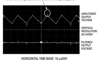
Figure 24. Output Ripple Voltage Waveforms
