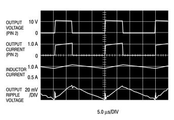
Figure 12. Switching Waveforms
