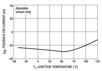
Figure 11. Feedback Pin Current
