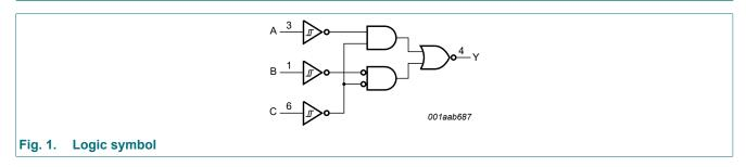
Low-power configurable multiple function gate
