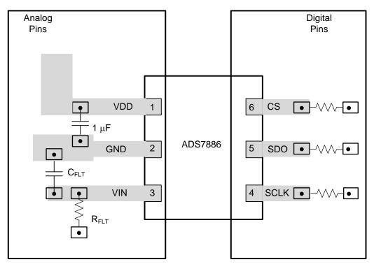
Figure 35. ADS7886 Layout Example
