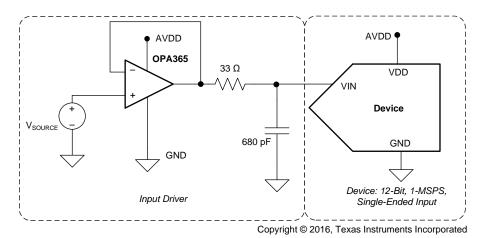
Figure 29. Typical Data Acquisition (DAQ) Circuit: Single-Supply DAQ
