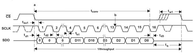
Figure 1. Interface Timing Diagram
