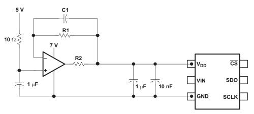
Figure 34. Buffering With the OPA735
