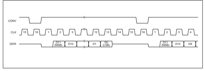
FIGURE 7. Typical DSP Interface Timing.
