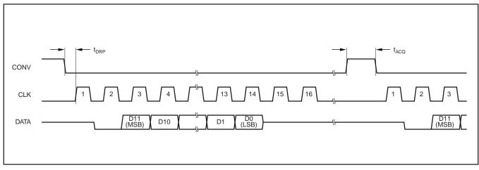
FIGURE 8. Typical SPI/QSPI Interface Timing.
