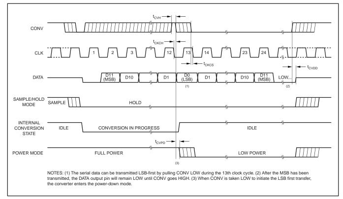
FIGURE 5. Serial Data "LSB-First" Timing.
