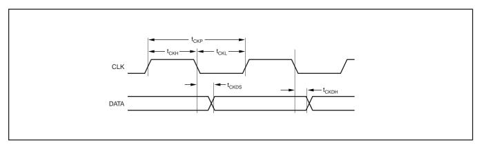
FIGURE 2. Serial Data and Clock Timing.
