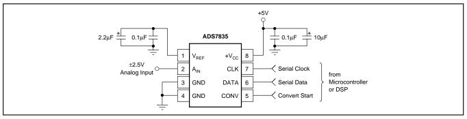
FIGURE 1. Basic Operation of the ADS7835.
