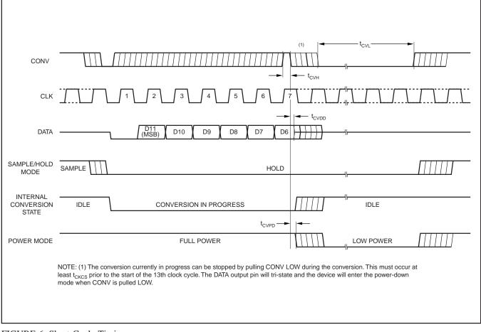
FIGURE 6. Short-Cycle Timing.
