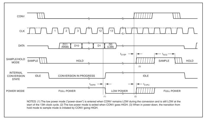
FIGURE 4. Power-Down Timing.
