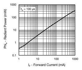
Fig. 6 - Radiant Power vs. Forward Current
