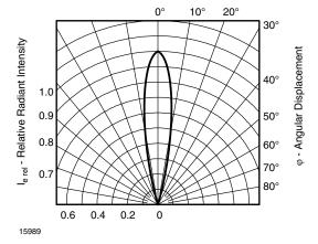
Fig. 9 - Relative Radiant Intensity vs. Angular Displacement
