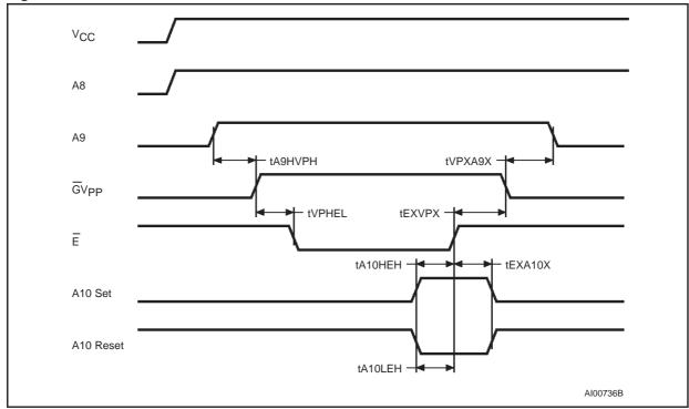
Note: A8 High level = 5V; A9 High level = 12V.
