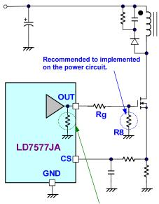
LD7577JA integrates an internal pull-low resistor to prevent any floating condition-
