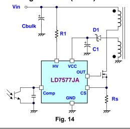
Traditional circuits' power on the PWM controller through a startup resistor to constantly provide current from a rectified voltage to the capacitor connected to Vcc pin. Nevertheless, this startup resistor was usually of larger resistance, and it therefore required more power and more time to start up.
