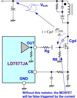
will be false triggered by the current through Cgd if Rg is disconnected.
