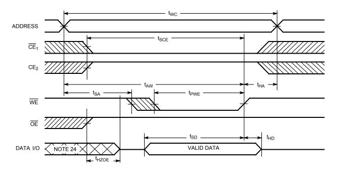
Write Cycle No. 2 ( $\overline{CE}_1$  or  $CE_2$  Controlled)[21, 22, 23]
