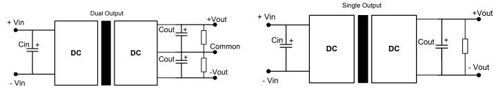
All the AM2LV-Z Series have been tested with the above recommended test circuit. This series should be tested under load.
