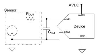
Figure 44. Interfacing the Device Directly with Sensors
