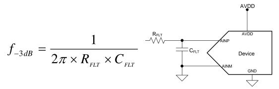
Figure 39. Antialiasing Filter
