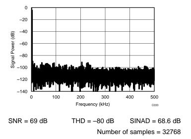
Figure 40. Test Results for the ADS7042 and OPA314 for a 2.5-kHz Input
