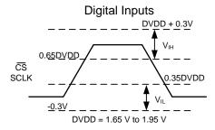
Figure 30. Digital Voltage Levels as per the JESD8-7A Standard
