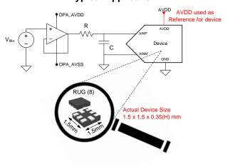
NOTE: The ADS7042 is smaller than a 0805 (2012 metric) SMD component.
