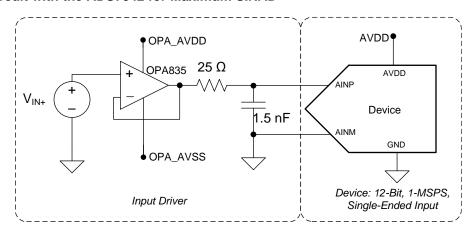
Figure 41. ADS7042 DAQ Circuit: Maximum SINAD for Input Frequencies up to 250 kHz
