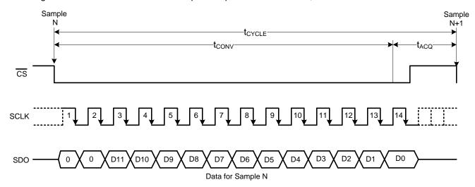
Figure 34. Serial Interface Timing Diagram
