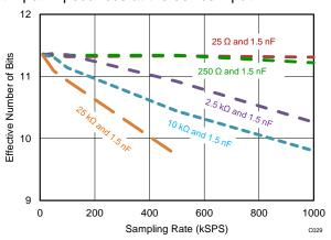
Figure 45. ENOB (Effective Number of Bits) Achieved from the ADS7042 at Different Throughputs
