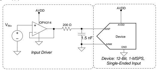
Figure 38. DAQ Circuit: Single-Supply DAQ
