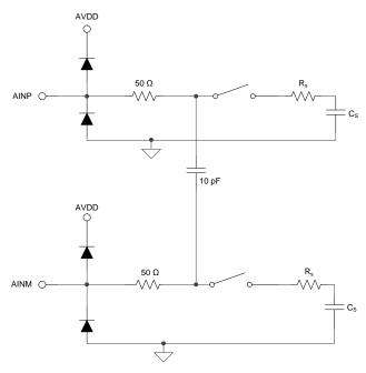
Figure 32. Equivalent Input Circuit for the Sampling Stage
