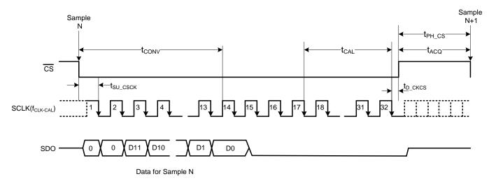
Figure 37. Offset Calibration During Normal Operation Timing Diagram
