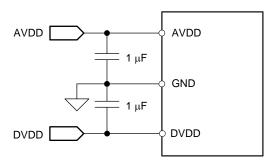
Figure 46. Power-Supply Decoupling
