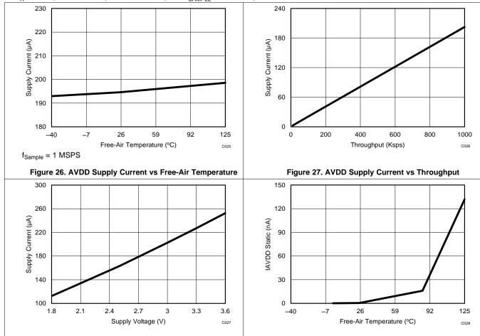
Figure 29. AVDD Static Current vs Free-Air Temperature
