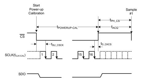
Figure 36. Offset Calibration on Power-Up Timing Diagram
