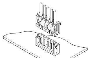
This, the thinnest, 2.5 mm pitch connector, is 8.1 mm in height after mounting and 3.8 mm in width. It is designed to meet the demand for the high-density connection of internal wires to printed circuit boards. It is compact, highly reliable and low in cost.
