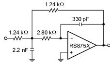
Figure 18. MFB 100 kHz 2<sup>nd</sup> Order Low-Pass Butterworth Filter Circuit
