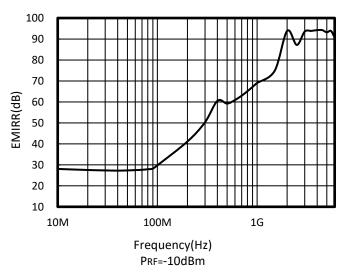
Figure 16.RS875X EMIRR vs Frequency
