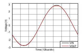
Figure 15. Output Waveform Devoid of Phase Reversal during an Input Overdrive Condition
