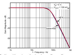
Figure 20. MFB and Sallen-Key 2<sub>nd</sub> Order Low-Pass Butterworth Filter Response
