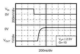
**Figure 13. Negative Overload Recovery**
