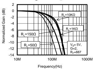
Figure 5. Frequency Response for Various RL
