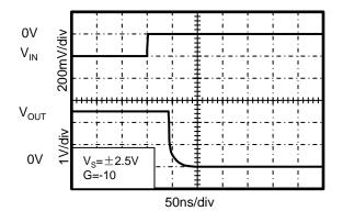
Figure 11. Large-Signal Step Response
