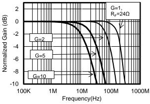
Figure 1. Non-Inverting Small-Signal Frequency Response
