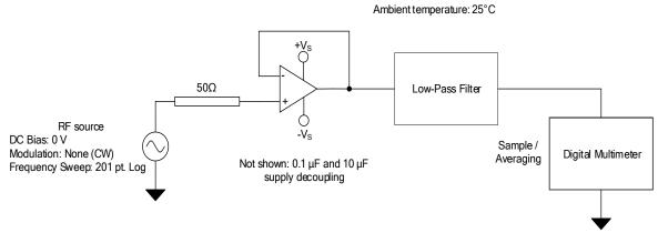
Figure 17. EMIRR IN+ Test Configuration Schematic
