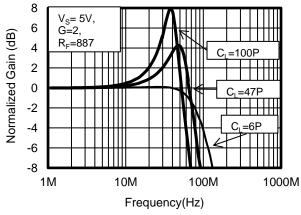
Figure 4. Frequency Response for Various CL
