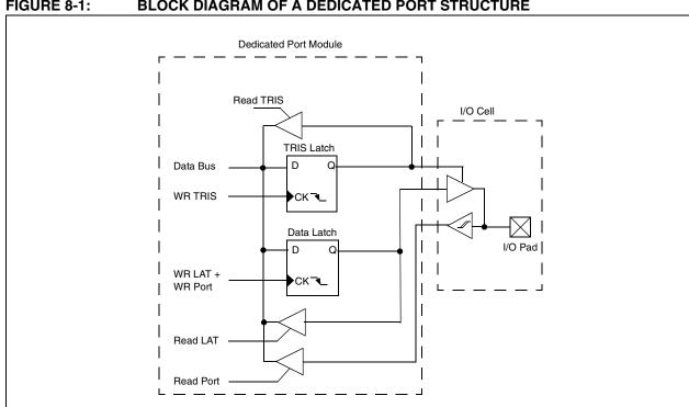
FIGURE 8-1: **BLOCK DIAGRAM OF A DEDICATED PORT STRUCTURE**
