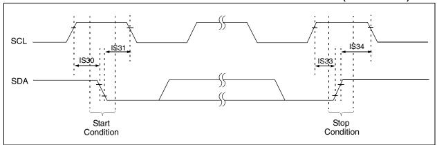
FIGURE 23-23: I<sup>2</sup>C™ BUS DATA TIMING CHARACTERISTICS (SLAVE MODE)
