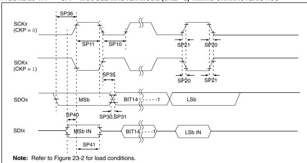
FIGURE 23-17: SPI™ MODULE MASTER MODE (CKE =1) TIMING CHARACTERISTICS
