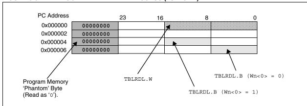
FIGURE 3-4: PROGRAM DATA TABLE ACCESS (MS BYTE)
