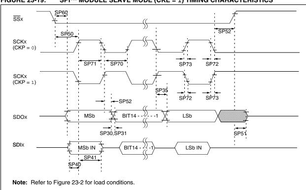
FIGURE 23-19: SPI™ MODULE SLAVE MODE (CKE = 1) TIMING CHARACTERISTICS
