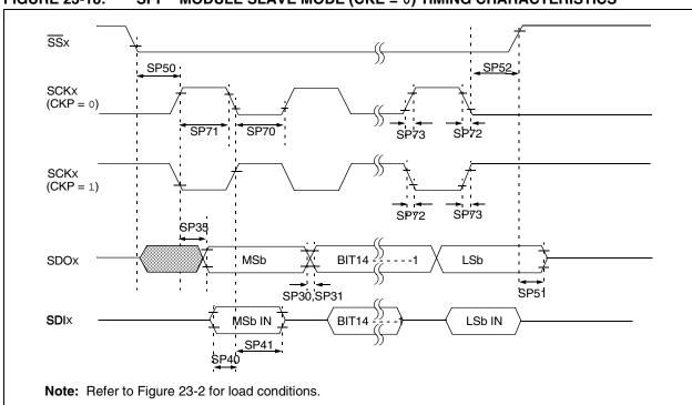
FIGURE 23-18: SPI™ MODULE SLAVE MODE (CKE = 0) TIMING CHARACTERISTICS
