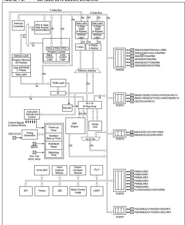
FIGURE 1-2: dsPIC30F3010 BLOCK DIAGRAM
