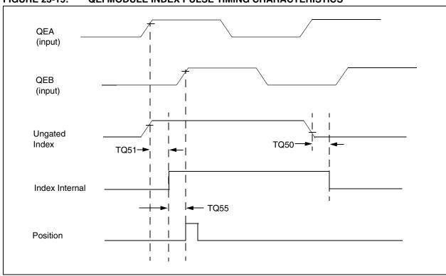
FIGURE 23-15: QEI MODULE INDEX PULSE TIMING CHARACTERISTICS
