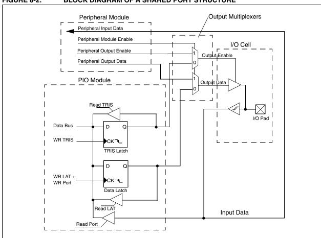
FIGURE 8-2: BLOCK DIAGRAM OF A SHARED PORT STRUCTURE
