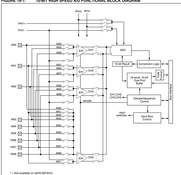
**FIGURE 19-1:** 10-BIT HIGH SPEED A/D FUNCTIONAL BLOCK DIAGRAM
