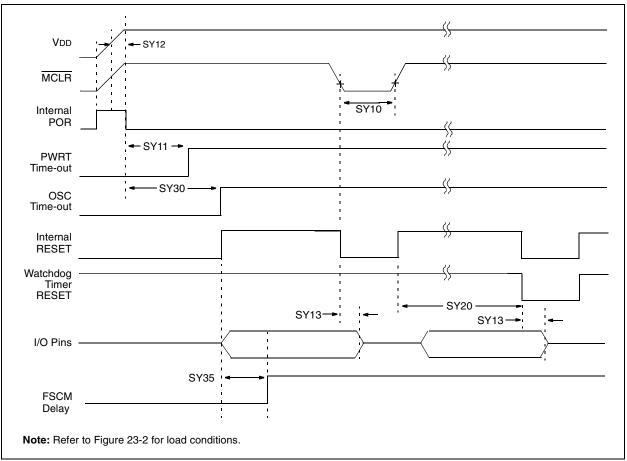
TABLE 23-20: RESET, WATCHDOG TIMER, OSCILLATOR START-UP TIMER, POWER-UP TIMER AND BROWN-OUT RESET TIMING REQUIREMENTS
