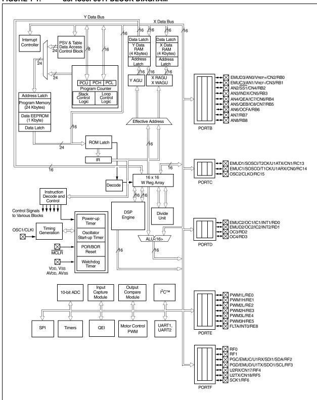
FIGURE 1-1: dsPIC30F3011 BLOCK DIAGRAM
