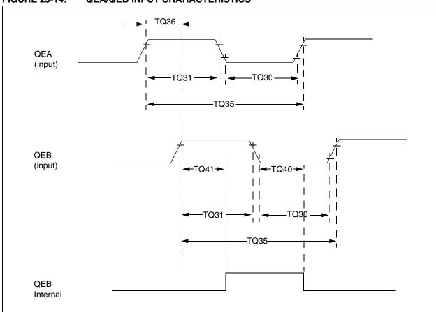
FIGURE 23-14: QEA/QEB INPUT CHARACTERISTICS
