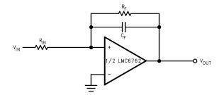
Figure 29. Canceling the Effect of Input Capacitance
