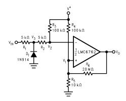
Figure 32. Zero Crossing Detector
