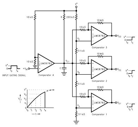
Figure 34. Time Delay Generator
