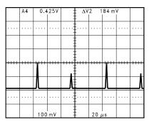
Figure 28. Measurement of the Shoot-Through Current
