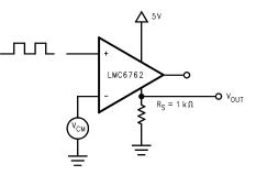
Figure 27. LMC6762 Circuit for Measurement of the Shoot-Through Current
