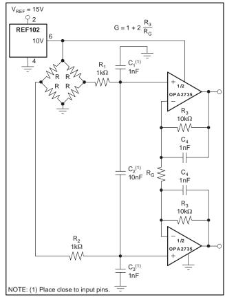
Figure 3. Differential Output Bridge Amplifier
