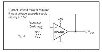
**Figure 1. Input Current Protection**
