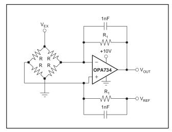
Figure 2. Single Op Amp Bridge Amplifier Circuit
