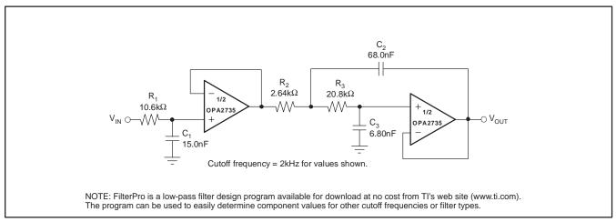
Figure 7. High DC Accuracy, 3-Pole Low-Pass Filter
