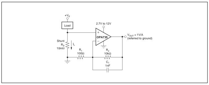
Figure 10. Low-Side Power-Supply Current Sensing
