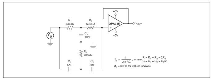
Figure 6. Twin-T Notch Filter
