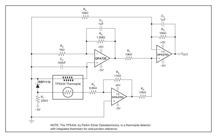
Figure 5. Thermopile Non-Contact Surface Temperature Measurement
