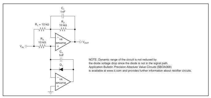
Figure 8. Precision Full-Wave Rectifier with Full Dynamic Range
