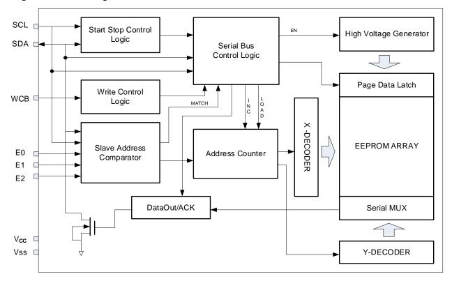
Figure 2-1 Block Diagram
