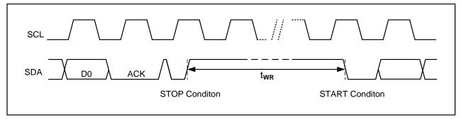
Note: [1] The write cycle time two is the time from a valid stop condition of a write sequence to the end of the internal clear/write cycle.
