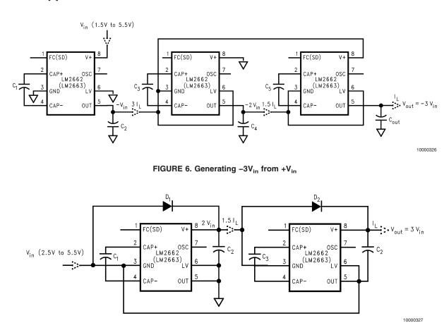
FIGURE 7. Generating +3V<sub>in</sub> from +V<sub>in</sub>
