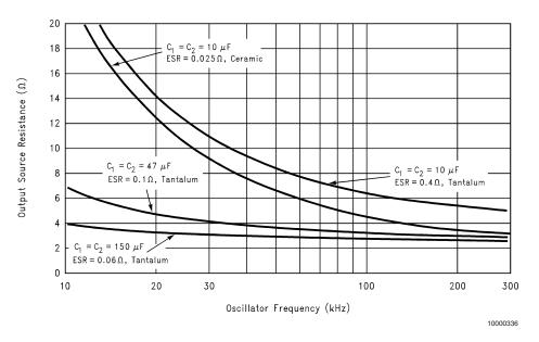
FIGURE 3. Output Source Resistance vs Oscillator Frequency
