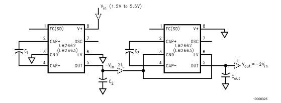
FIGURE 5. Increasing Output Voltage by Cascading Devices
