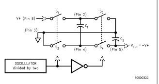
FIGURE 2. Voltage Inverting Principle
