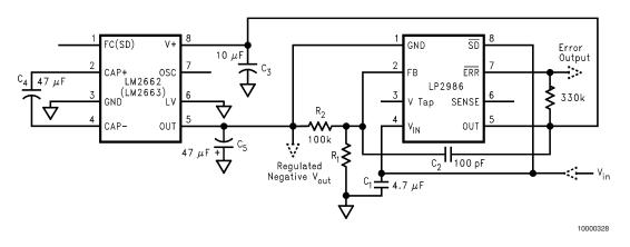
FIGURE 8. Combining LM2662/LM2663 with LP2986 to Make a Negative Adjustable Regulator
