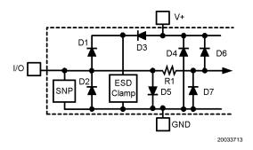
FIGURE 1. ESD Protection Input Structure
