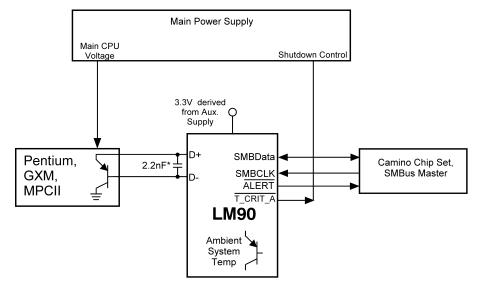
\*Note: 2.2nF Capacitor must be placed as close as possible to D+ and D- pins of the LM90.
