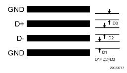
FIGURE 15. Ideal Diode Trace Layout
