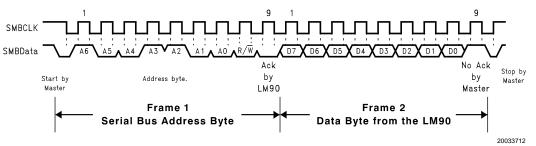
(c) Serial Bus Read from a Register with the Internal Command Register preset to desired value.
