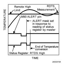
FIGURE 4. ALERT Output as an Interrupt Temperature Response Diagram
