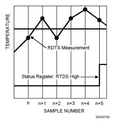
FIGURE 10. Fault Queue Temperature Response Diagram
