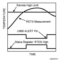
FIGURE 3. ALERT Comparator Temperature Response Diagram
