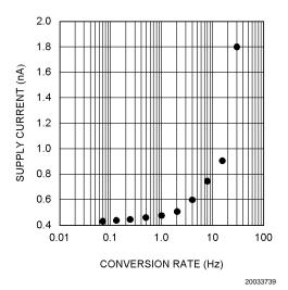
FIGURE 2. Conversion Rate Effect on Power Supply
