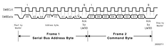
(b) Serial Bus Write to the Internal Command Register
