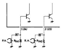
The difference in the value between  $R_{\rm IN}1$  and  $R_{\rm IN}2$  causes the variation in amp output DC voltage at the time of F/R switching. Therefore, the input DC voltage (voltage across  $R_{IN}$ ) must be made as equal as possible.
