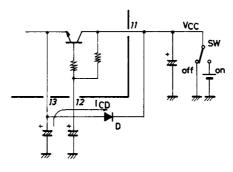
(6) The output MIX circuit is of the emitter follower configuration as shown below.
