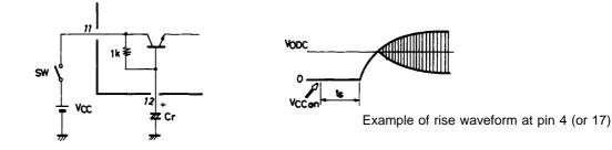
When supply voltage  $V_{CC}$  is switched ON, the amplifier output (pins 4, 17) will rise. Output waveform ON time  $t_s$  can be varied by capacitor Cr connected to pin 12.
