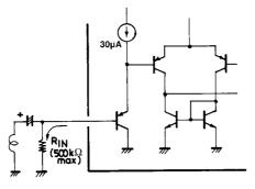
If a resistor of more than  $500 \text{ k}\Omega$  is connected across input pin and GND, the noise (output) caused by amp 1 and amp 2 select is liable to increase at the time of F/R switching.
