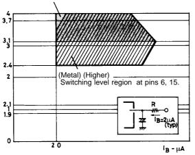
Switching level (reverse) on pin 9 at V\_{CC} = 6.0 V, Ta = 25°C
