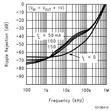
Ripple Rejection (V<sub>IN</sub> = 5.0V)
