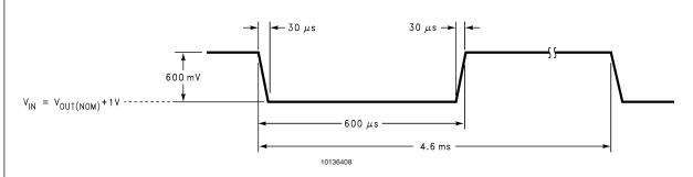
FIGURE 1. Line Transient Input Test Signal
