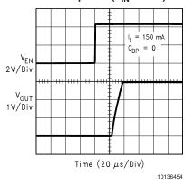
Enable Response ( $V_{IN} = V_{OUT} + 0.2V$ )
