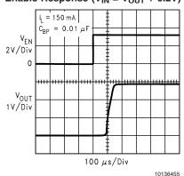
Enable Response ( $V_{IN} = 4.2V$ )
