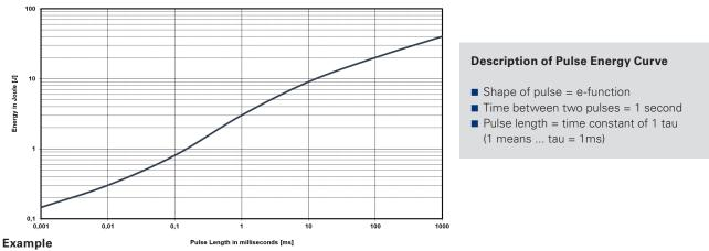
At 1 ms tau the LXP-20 with e.g. 1  $\Omega$  to 10  $\Omega$  can withstand an energy level of about 3 J, when the pulse pause time is  $\geq$  1s
