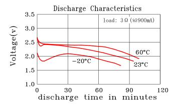
Discharge characteristics on temperature
