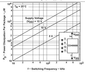
Figure 6. Power Dissipation per Package vs Switching Frequency
