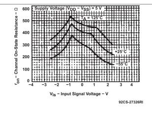
Figure 1. Typical ON-State Resistance vs Input Signal Voltage (All Types)
