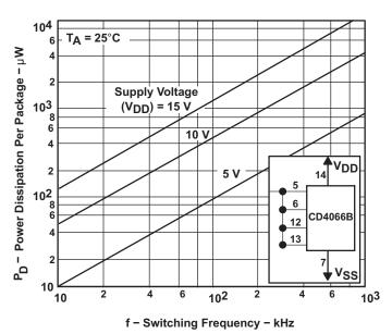
Figure 19. Power Dissipation vs. Switching Frequency
