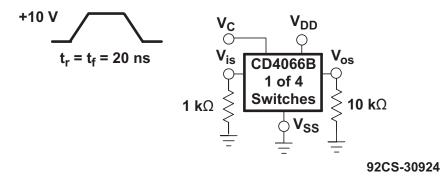
All unused terminals are connected to V<sub>SS</sub>.
