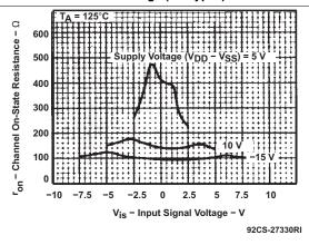
Figure 4. Typical ON-State Resistance vs Input Signal Voltage (All Types)
