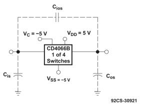
Measured on Boonton capacitance bridge, model 75a (1 MHz); test-fixture capacitance nulled out.
