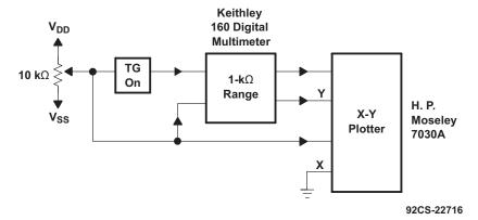
Figure 8. Channel On-State Resistance Measurement Circuit
