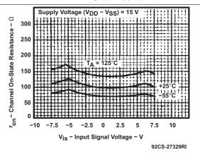
Figure 3. Typical ON-State Resistance vs Input Signal Voltage (All Types)
