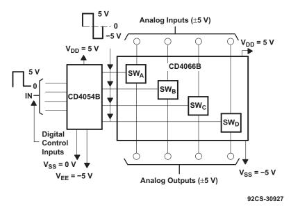
Figure 18. Bidirectional Signal Transmission Through Digital Control Logic
