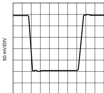
Figure 37. Non-Inverting Large Signal Pulse Response
