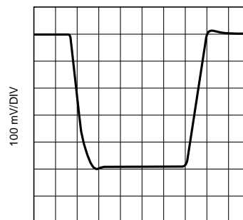
Figure 38. Non-Inverting Large Signal Pulse Response
