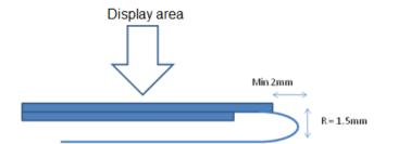
(12) The module should be fixed balanced into the housing, or the module may be twisted.
