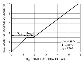
Figure 8. Gate-to-Source vs. Total Charge
