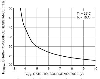
Figure 3. On-Resistance vs. Gate-to-Source Voltage
