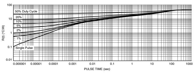
Figure 13. Thermal Characteristics
