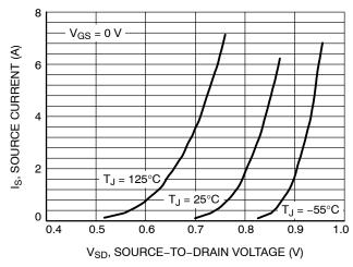
Figure 10. Diode Forward Voltage vs. Current
