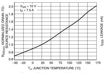
Figure 5. On–Resistance Variation with Temperature
