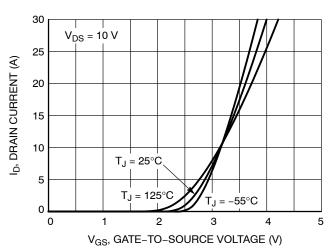
Figure 2. Transfer Characteristics
