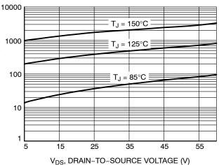
Figure 6. Drain-to-Source Leakage Current vs. Voltage
