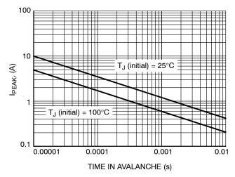
Figure 12.  $I_{\mbox{\scriptsize PEAK}}$  vs. Time in Avalanche
