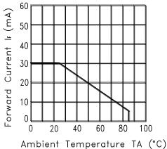
Fig.3 FORWARD CURRENT DERATING CURVE
