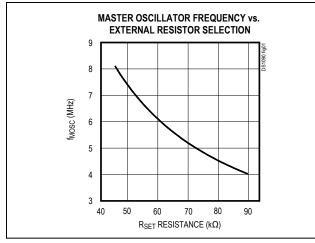
Figure 1. Master Oscillator Frequency
