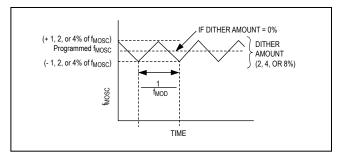
Figure 2. Center Frequency Dither Diagram
