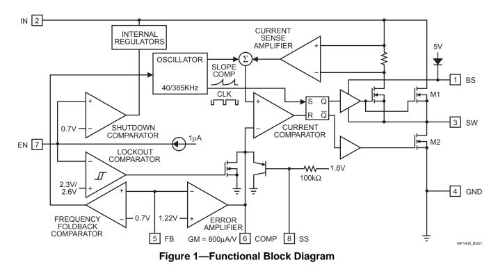
The MP1430 is a current-mode step-down regulator. It regulates input voltages from 6V to 28V down to an output voltage as low as 1.22V, and is able to supply up to 3A of load current.
