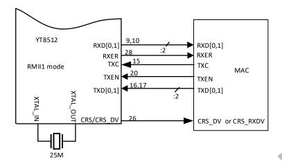
Figure .connection diagram of RMII1(with 25MHz and 50MHz clock)
