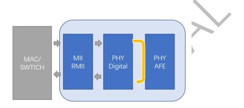
Figure . Internal loopback
