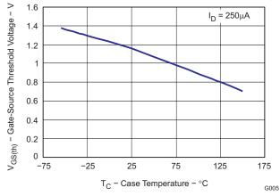
Figure 6. Threshold Voltage vs. Temperature
