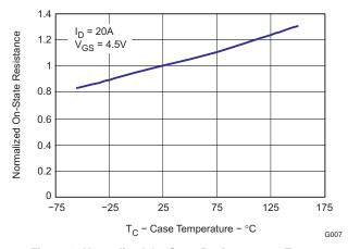
Figure 8. Normalized On-State Resistance vs. Temperature
