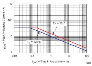
Figure 11. Single Pulse Unclamped Inductive Switching
