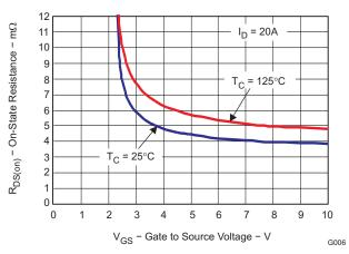
Figure 7. On-State Resistance vs. Gate to Source Voltage
