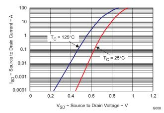
Figure 9. Typical Diode Forward Voltage
