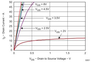
Figure 2. Saturation Characteristics
