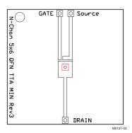
Max  $R_{\theta JA} = 123^{\circ} C/W$  when mounted on minimum pad area of 2-oz. (0.071-mm thick) Cu.
