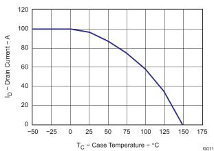
Figure 12. Maximum Drain Current vs. Temperature
