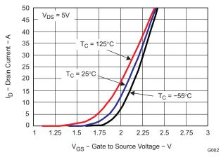
Figure 3. Transfer Characteristics
